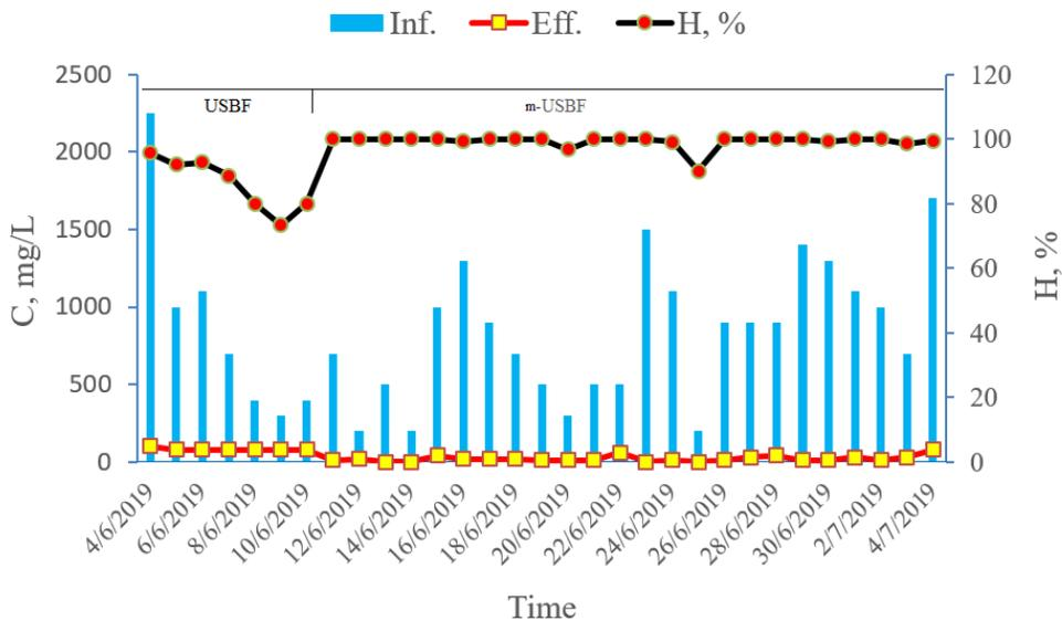
**Figure 3.** Suspended solids (SS) removal.
