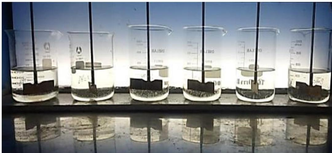
**Figure 2.** Jar-test procedure.
