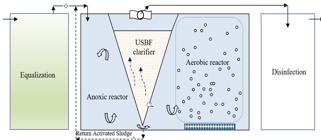
Figure 1. USBF bioreactor of Le Meridien Saigon Hotel.
