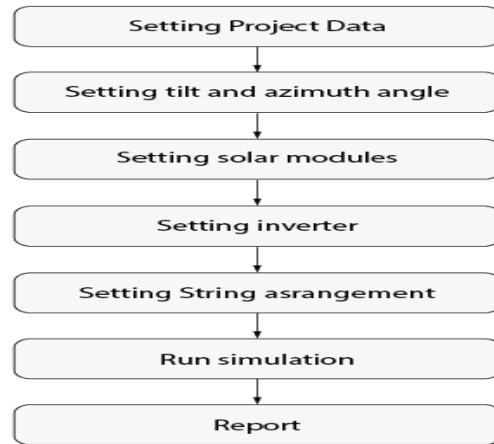
Figure 10. Process of simulation and design in PVyst software
