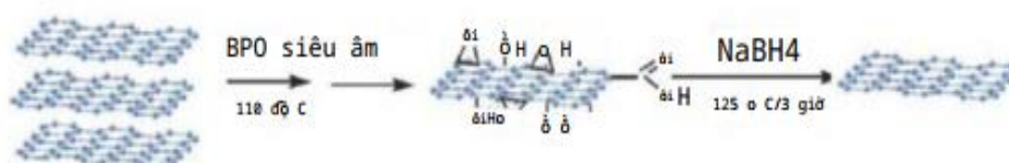
Figure 4. Synthesis of graphene from BPO (Tong et al., 2013)
