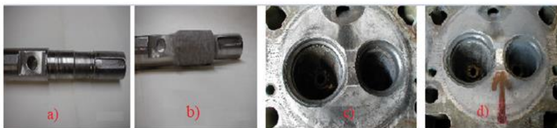
Figure 7. Examples of restoration of geometric dimensions and properties of products: a, b – recovery of abrasive shaft c, d – removal of cracks in cast iron engine
