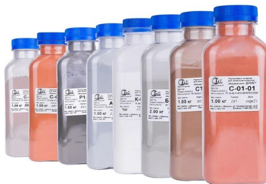
Figure 5. The metal powder used in CGDS technology
