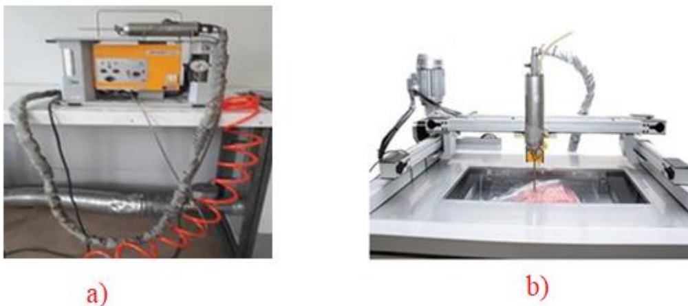
Figure 3. Equipment for applying CGDS: a – manual device; b– automated complexes
