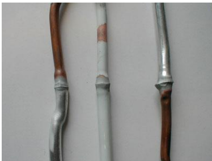
Figure 8. Hermetic connection of a copper tube with an aluminum one
