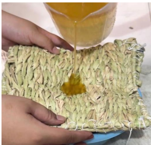
Figure 4. The water hyacinth pad absorbs oil residue and is tested for its ability to absorb oil
