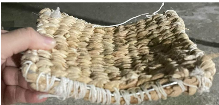
Figure 2. Water hyacinth pad product absorbs cooking oil scum completely
